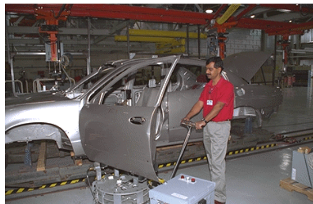
Cobots & Intelligent Assistance Devices at General Motors in 1998: Making robots work with the line worker.
